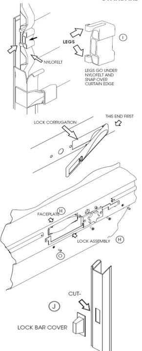
Lock Bar Cover must be installed to prevent finger
