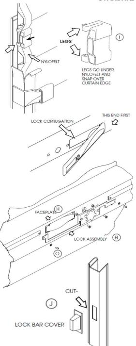
Lock Bar Cover must be installed to prevent finger
