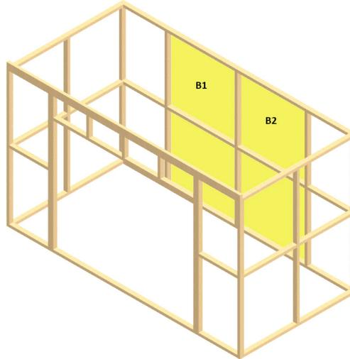
The above image shows the possible positions for PA doors. After selecting the desired position(s), use the dimensions specified in the following image to make PA door slope.
